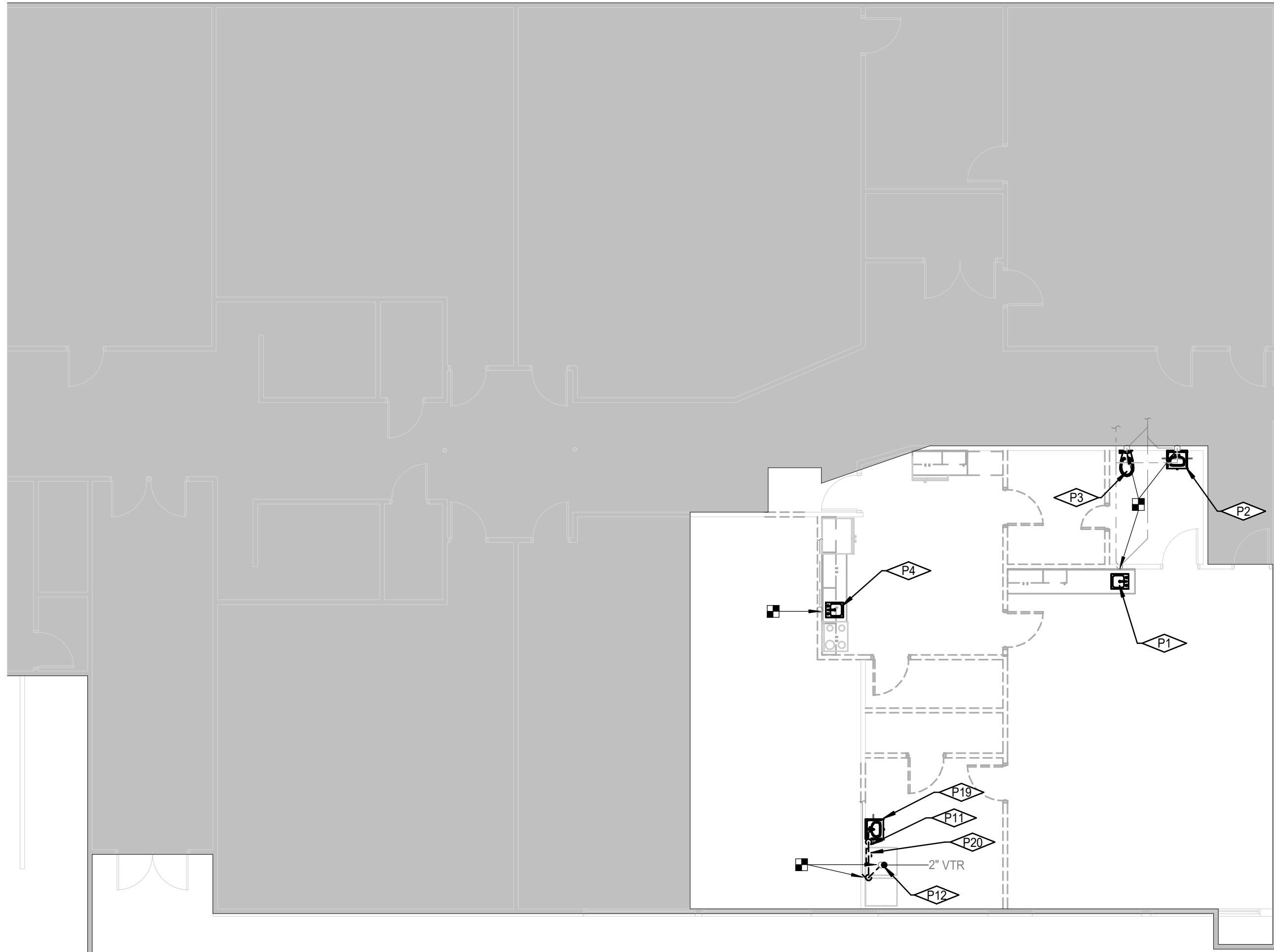
LEVEL 1 WASTE & VENT DEMOLITION PLAN SCALE: 1/8" = 1'-0"
